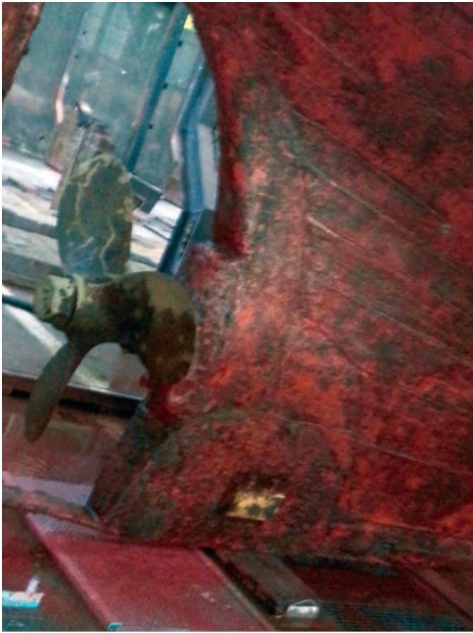
Fig. 1 — A bronze alloy propeller before (dirty/silver colored) and after (gold/copper colored) drydock restoration on a nearly 100-year-old wooden boat that's still used for fishing in Alaska.
