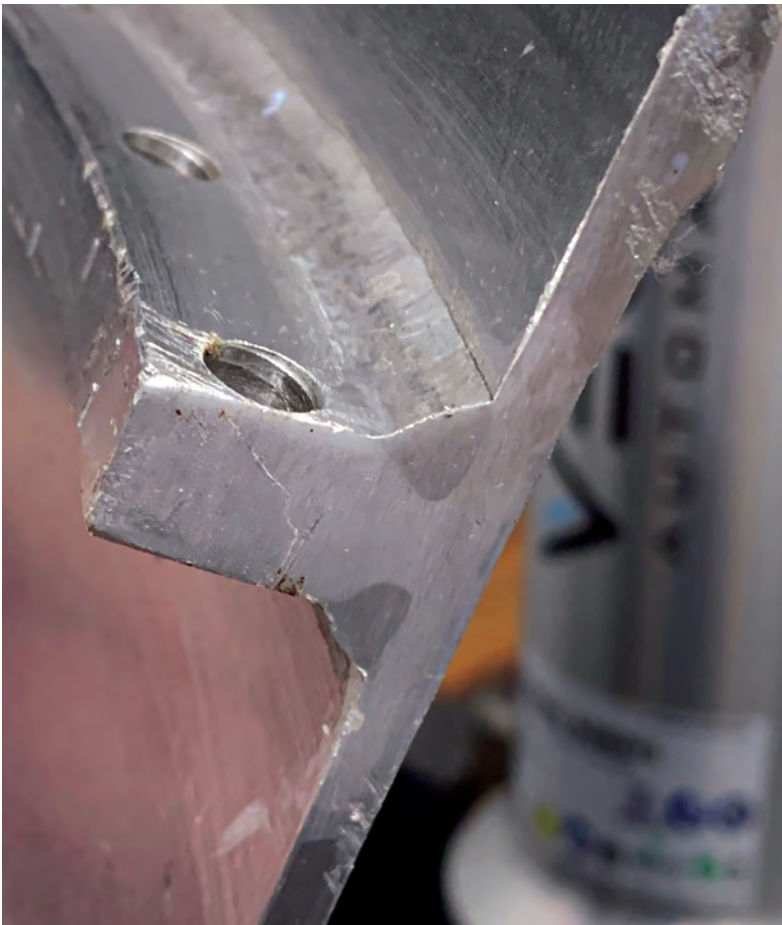
Fig. 1 — The Vectis applications engineering team used a tight, crisp arc paired with a heavy push angle to achieve both deep penetration and an ideal bead profile.
