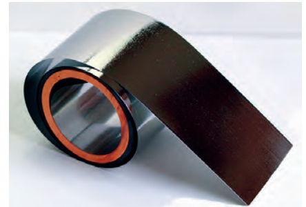
Fig. 1 — Amorphous foil TiBraz620 to form NbTi and NbZr superconducting phases after brazing.
