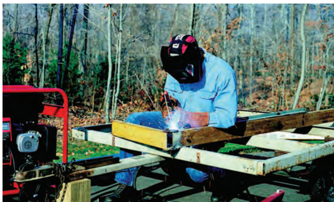
Fig. 1 — In some cases, natural air movement provides enough ventilation and fresh air to protect against overexposure to gases and fumes. (Photo credit: AWS Welding Handbook, Ninth Edition, Volume 2, Welding Processes, Part 1.)
