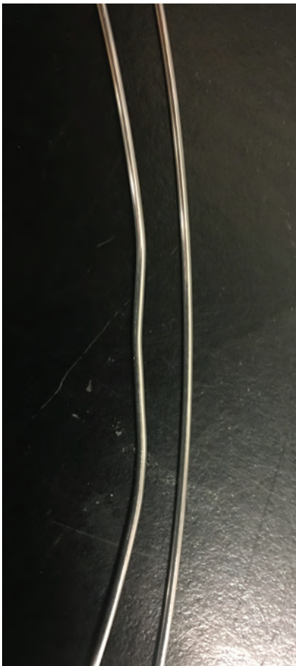
Fig. 3 — Even subtle bends in the wire can cause feeding issues as the wire passes through the contact tip.
