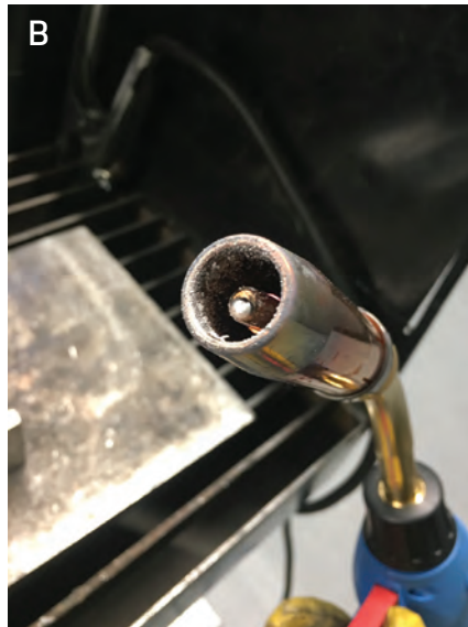
Fig. 4 — A — Buildup from arcing in the contact tip caused by lack of connectivity; B — the ever so familiar view that a welding operator has after suffering a burnback.
