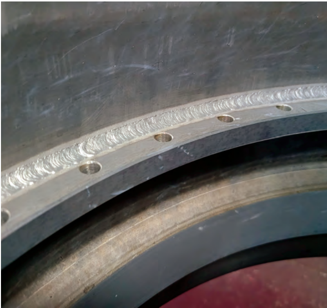
Fig. 3 — A close-up of the live welding shown in the lead photo.
