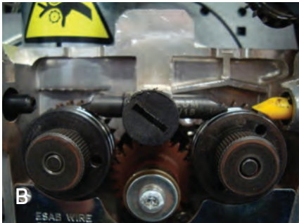
Fig. 6 — A — Pictured is how welding feeder equipment is commonly configured. Note the steel guides and space between the guides and the drive wheels; B — a welding feeder optimized for feeding softer aluminum wire. Note the nylon guides and the proximity to the drive wheels.
