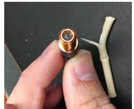
Fig. 8 — Shavings built up from severe rubbing on the inlet of a contact tip.
