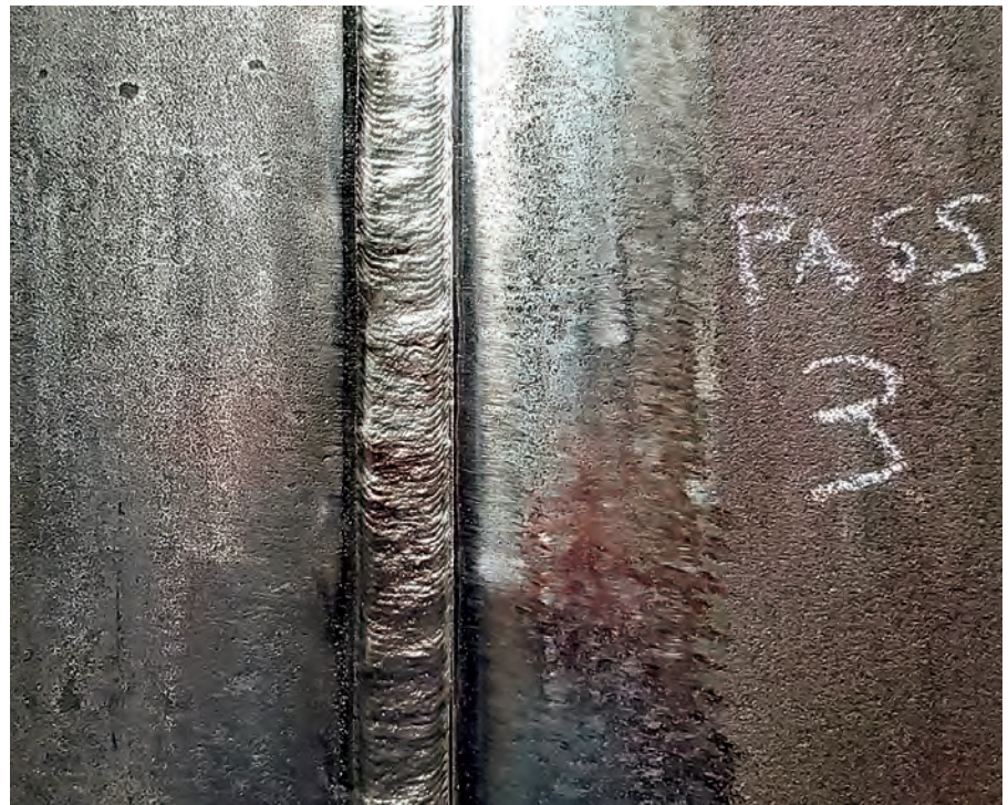
Fig. 4 — Bead profile of an enhanced ENiCrMo-4Ti-1/-4 in the 3G position with automated welding.
