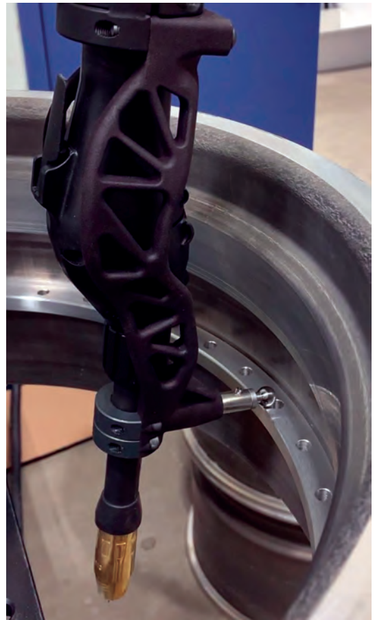
Fig. 2 — The touch probe leverages a 3D printed design and Vectis's unique force-based Touch Sensing feature to accommodate the wide variety of SRS custom rims.
